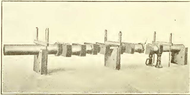
FIG. 30.—Fracture in Web Cut Away for Welding a Crankshaft.
